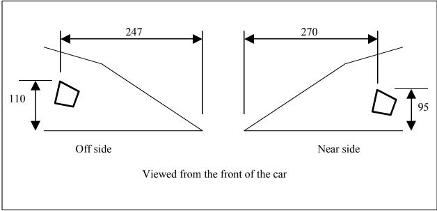
The dimensions are for the position of "T", the top of the shape. Measure horizontally from the inside point of the headlamp face. Measure vertically from the bottom edge of the headlamp face. For best results I find the left hand edge of the shape (viewed from the front) is nearly vertical.
