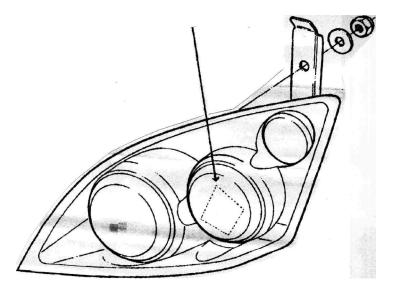
The detail came from the Lotus – Skipton Project (alias VX220). They said "Use black tape – similar to stick on number plates). Remove from lamp as soon as convenient to avoid possible damage / melting of tape / lamp."
