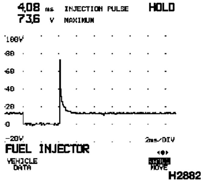
This multi-point fuel injection system is a conventional fuel injection system with a cut-off control system. In this case, the signal plot only has one voltage spike.
