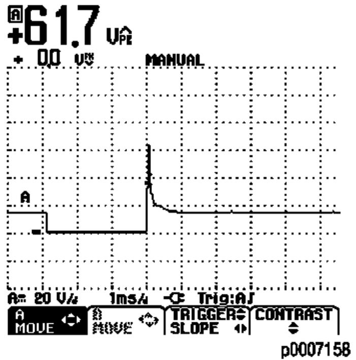
This multi-point fuel injection system is a conventional fuel injection system with a cut-off control system. In this case, the signal plot only has one voltage spike.
