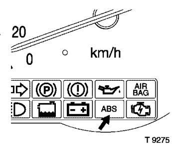
Conventional braking becomes operative if the ABS malfunctions. The trouble codes can be read using TECH 2.
