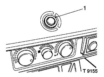
A pushbutton switch (1) is located in the steering column cowl to reset the odometer to zero and to control the brightness of the instrument illumination.
