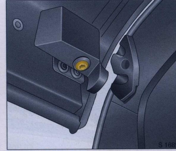
7. Unscrew the bolt that secures the rear cup bracket and remove the bracket.
