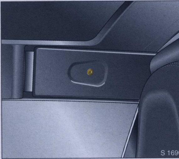
5. Unscrew the bolt that secures the rear cover panel and remove the panel.
