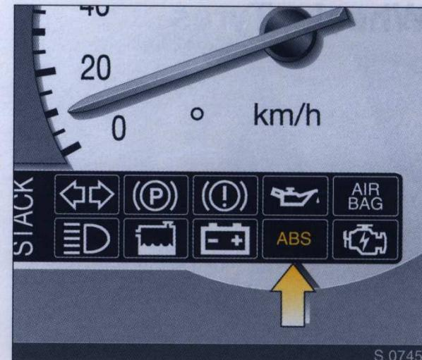
When the ignition is switched on, the ABS control indicator lights up. At the same time, the system performs a self-check which may be audible. When the control indicator goes out the system is ready for operation. If the control indicator does not go out after a few seconds, or if it lights up during driving, there is a fault in the ABS. The vehicle's brake system remains operational without ABS regulation.
