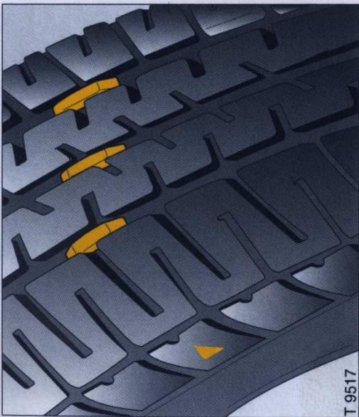
For safety reasons, tyres should be replaced when their tread depth has worn down to 2-3 mm. The legal permissible minimum tread depth (1.6 mm) has been reached when the tread has worn down as far as one of the wear indicators.
