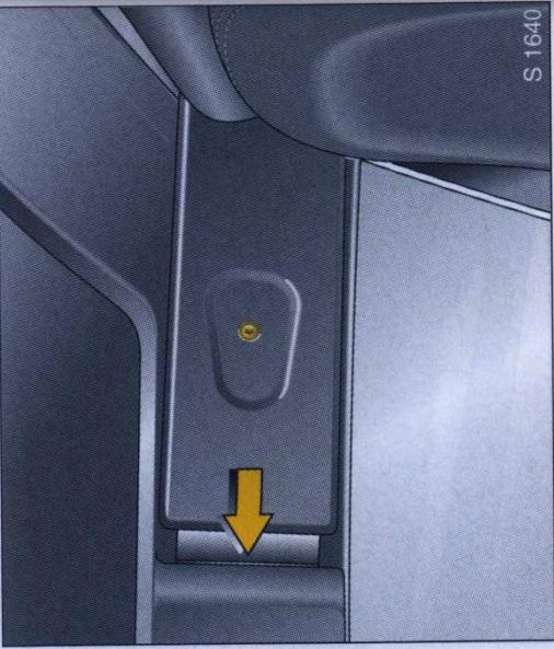
The rear cover panels are hinged and can only be installed to their respective sides.
