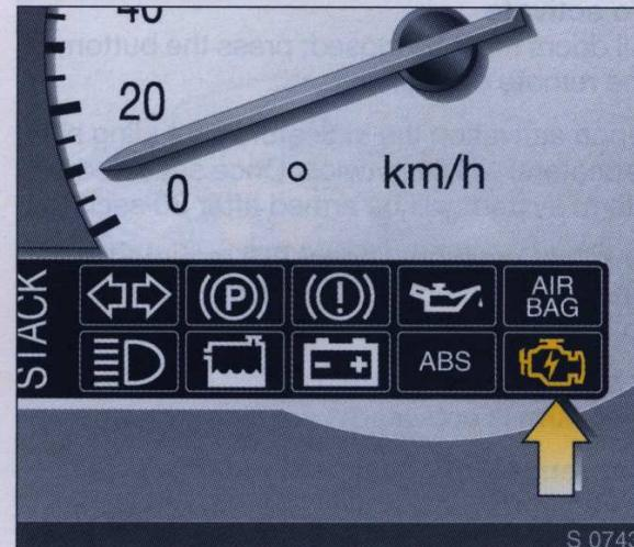
The control indicator lights up when the ignition is switched on then goes out.
