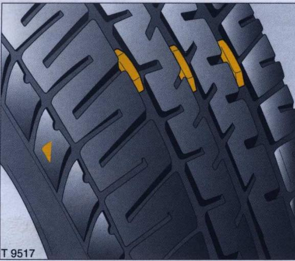
For safety reasons, tyres should be replaced when their tread depth has worn down to 2-3 mm. The legal permissible minimum tread depth (1.6 mm) has been reached when the tread has worn down as far as one of the wear indicators.
