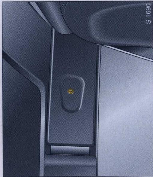
5. Unscrew the bolt that secures the rear cover panel and remove the panel.
