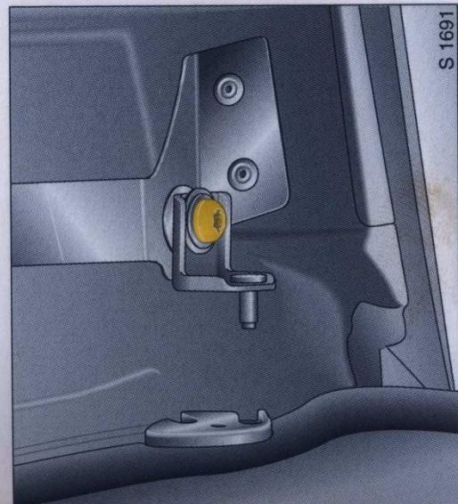
3. Unscrew the bolt that secures the front dowl bracket and remove the bracket.
