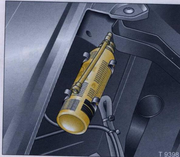
Screw the aerosol tube on to the tyre valve and remove the cap. Hold the can upright and press the button, holding until the tyre is fully inflated.
