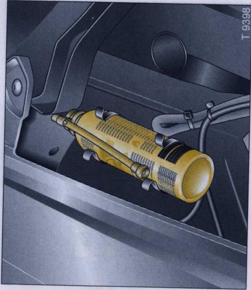
Screw the aerosol tube on to the tyre valve and remove the cap. Hold the can upright and press the button, holding until the tyre is fully inflated.
