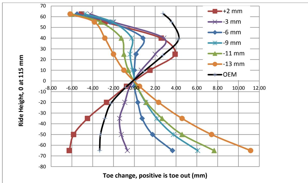
The numbers indicate the height of the pivot point with regards to the OEM steering arm. So -3 mm means 3 mm lower. OEM is OEM height of the pivot point. The rack is raised, using the 10 notch riser plates. Beware that at higher bump values the track rod started to hit the adjustable steering arm, forcing it down. This causes all the curves to convert to one point.
