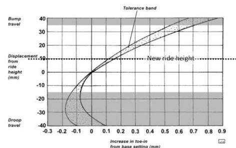
Now lowering the car 10 mm means another part of the curve is important. The interval changes with ride height and you have to deal with another part of the curve. With this curve, lowering the car is not much of an issue. At least not for bumpsteer. The relevant part of the curve doesn't change much.
