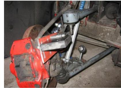
Although I made it from pretty solid material, what happened is that at maximum bump, the track rod hit the plate that holds the track rod end. After seeing the curves and wondering about how they converged, I had a look at the plate and found a sizeable dent in it. So measurements at high bump values are not valid.
