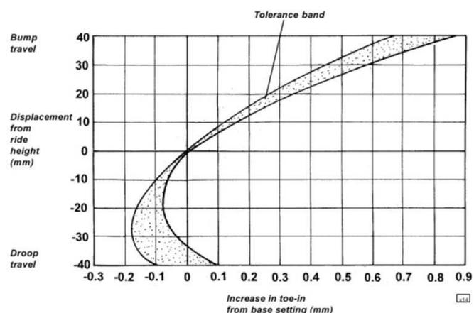
ride height changes from 115 to 110 mm, but the origin on the y-axis remains the same. If with those wheels the actual ride height is not 110 but 120 mm, the new origin on the y-axis will be at -10 mm.
