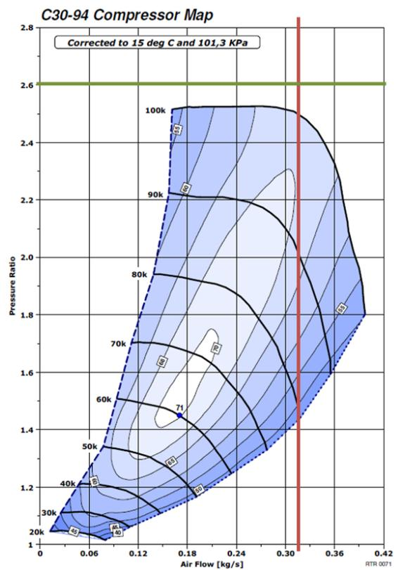
Off the map, but seems likely the TVS1320 can cope with a flow of 0.32 kg/sec at a PR of 2.6, but efficiency will suffer
